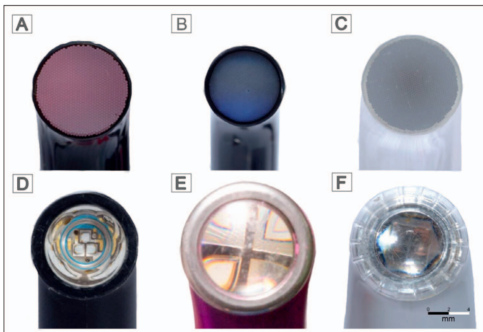
Figure 2. LED light-curing tips. (A): Bluephase Style. (B): ESPE Cordless. (C): Elipar S10. (D): Demi Ultra. (E): Valo Cordless. (F): Radii-Cal. Note the different tip diameters (all tips imaged to the same mm scale).
